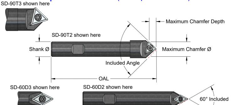
\*These all use Industry Standard inserts with secondary clearance facets ground to avoid dragging on the small cut diameters.\*
