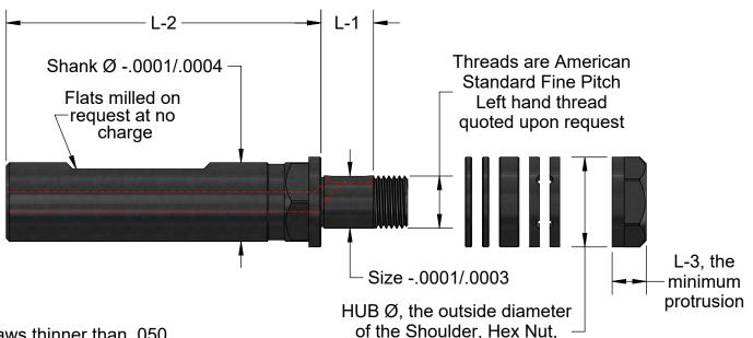
Saws thinner than .050 must not rest on the shoulder. Either on one spacer or several
