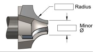
All AB Tools corner rounders are made with these features to avoid gouging.
