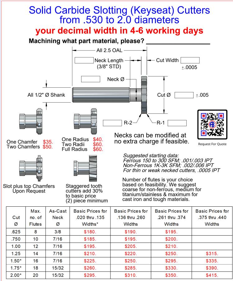
\*1.50 Cut Dia. Minimum width .050, 1.75 - 2.00 Cut Dia. Minimum width .060
