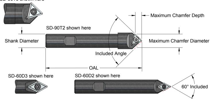
\*These all use Industry Standard inserts with secondary clearance facets ground to avoid dragging on the small cut diameters.\*
