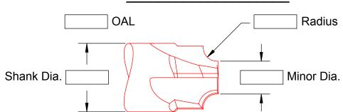
All AB Tools corner rounders are made with these features to avoid gouging.
