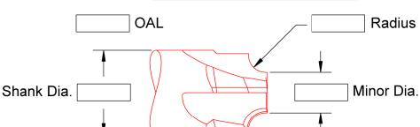
All AB Tools corner rounders are made with these features to avoid gouging.
